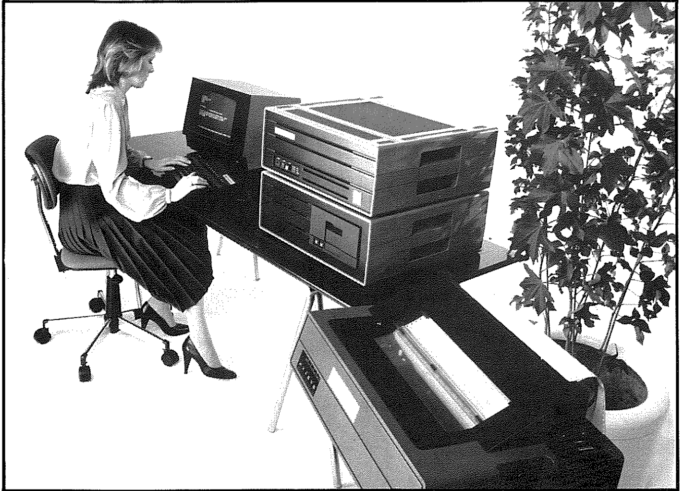
The GEC 4150 central processor (top) with 8" disc drive unit
